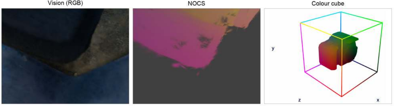
Figure 3.1: The NOCS encoding. Left: the close-up vision image of a contact region. Centre: the corresponding nocs image, where each pixel’s RGB colour is the normalized 3D position (Eq. 3.2) of the scene point it observes. Right: the unit cube illustrating the mapping: the x, y, z axes are tinted by the matching RGB channels and the object is coloured by its position inside the normalized scene box.
